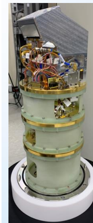
Cold cartridge assembly (ASTE 275-500 GHz Rx)
